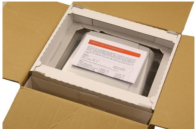
Fig 2: Top padding with membrane facing down to squeeze monitor in the middle.
