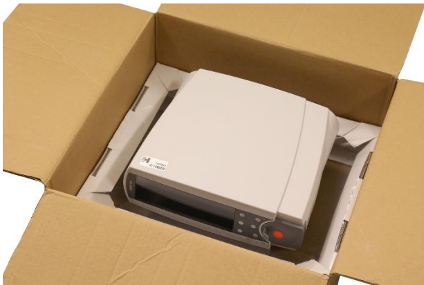
Fig 1: Monitor placed on bottom padding with membrane facing up.
