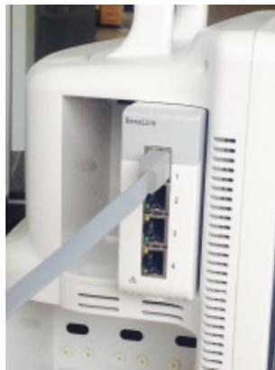
4. Connect the free end of the RJ45 Cable to the BeneLink ID Adapter (grey box).
