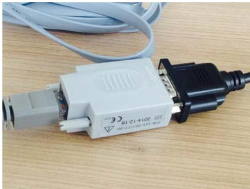
5. Use the Mindray type C serial port adapting cable (black cable) to connect the ID-Adapter with the female RS-232 connector on the rear of the SDM.
