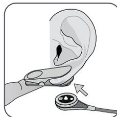
**9.** Pull the earlobe with the Ear Clip in horizontal position. Move the sensor horizontally into place with the cable preferably pointing to the crown of the head. Insert the sensor into the clip's retainer ring by gently pressing it until it snaps into the clip.
