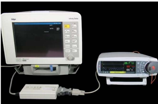
6. Switch the Dräger Medical patient monitor ON and select  $tpCO_2$  and  $tpO_2$  parameter on the Dräger Medical patient monitor (refer to corresponding patient monitor configurations manual).
