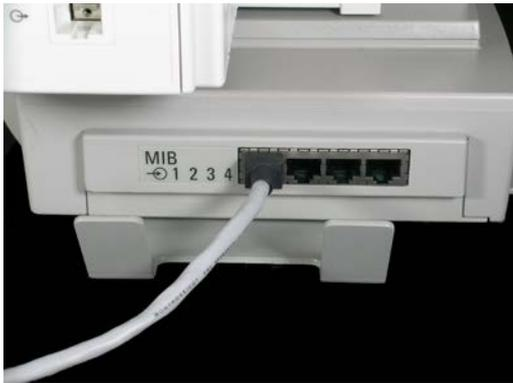
3. Connect the MIB II Converter to MIB Connector using the Patch Cable.
