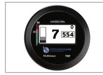
The Digital Multimeter (DM) has six different operating modes: POST, Wake, Active, Report, Sleep, and Fault.
