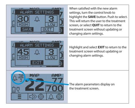
**NOTE:** The process is the same for setting both high and low alarms. **NOTE:** The alarm setting will not change if the user presses **EXIT** before confirming the change.
