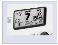
The treatment screen displays Amplitude, Mean Airway Pressure, Frequency, alarm high and low setpoints, battery condition, charging status, and power plug indicator.
