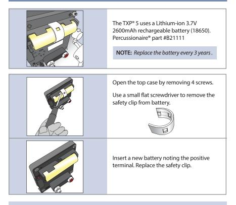
**NOTE:** Ensure the battery is fully charged before storing the TXP<sup>®</sup> 5. **NOTE:** Only use batteries provided by Percussionaire<sup>®</sup>. **Do not use batteries from other manufacturers.**
