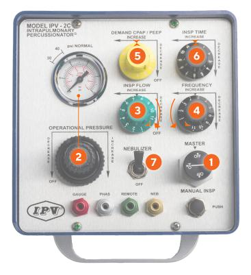
Master Switch turns the IPV®-2C controller ON and OFF.
