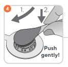
Holding the sensor at its neck, approach the MAR/e and first insert the nose of the sensor into the ring. Click in the sensor by applying slight downward pressure on its neck. Rotate the sensor in the ring into the best position and press the sensor gently against the skin to spread the Contact Gel. Verify that air gaps between the skin and the sensor are eliminated and that the sensor can easily be rotated.
