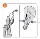
Remove the protective films on the ear clip and attach the clip to the earlobe with the retainer ring on the back or the earlobe. Ensure that the skin beneath the clip is not wrinkled and that the hole in the center of the ring completely covers the skin.
