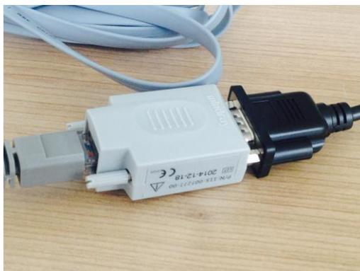
5. Use the Mindray type C serial port adapting cable (black cable) to connect the ID-Adapter with the female RS-232 connector on the rear of the tCOM+.
