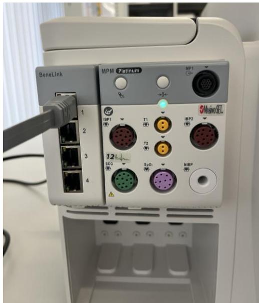
4. Connect the free end of the RJ45 Cable to the BeneLink ID Adapter (grey box).
