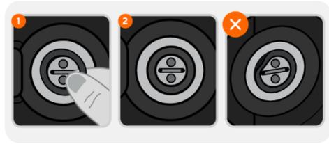
2. Place a new Gasket onto the groove of the Docking Station, gently press around the circumference of the Gasket to push it into the groove, using thumb or finger. Note that the calibration chamber (in the center of the Docking Station) has a suspension mechanism and may therefore be pushed inwards without any risk to the monitor.
