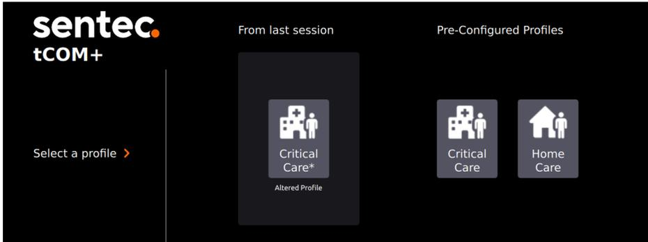
To be able to continue, users must choose one of the profiles depicted. If the connected sensor is in the Docking Station, 'Calibration in progress' or 'Ready for use' is displayed in the center of the screen.
