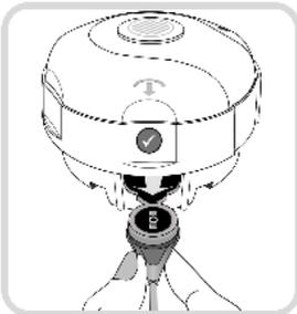
Press one last time or lift the sensor and remove it from the Membrane Changer. The ✓ symbol indicates that the membrane change is completed.
