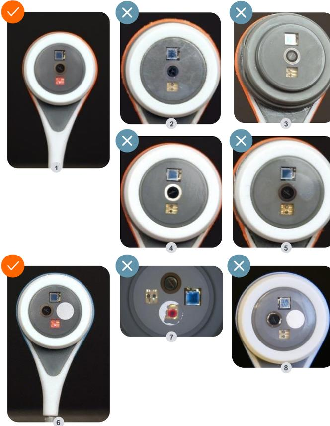
**Checking a V-Sign™ Sensor (see image 1 above):** Look for a smooth, clear membrane without scratches or air bubbles. The center ring should be a shade of brown to black and the red LED light should be on when connected to the monitor.
