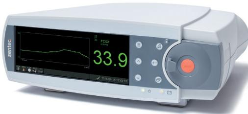
Sentec Connectivity enables the transmission of oxygenation and ventilation monitoring – **tcPCO<sub>2</sub>, SpO<sub>2</sub>, Pulse Rate (PR)** – to EOVE EO-150 Ventilator.
