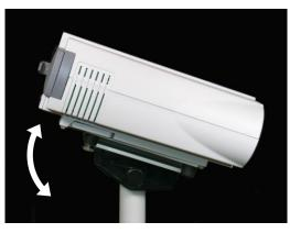
**6)** You may adjust the pivoting head for a better viewing angle. Loosen the two screws of the pivoting head and push the appliance carefully into the desired position. Then fix the plate in the desired position and fasten the screws of the pivoting head.
