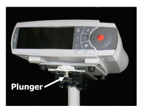
**5)** Attach the SDM to the Roll Stand by sliding the mounting plate as far as it will go into the appliance and until the plunger snaps in accompanied by a clicking sound.
