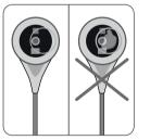
a) Change the sensor membrane if it is damaged or missing, has a loose fit, or if there is trapped air or dry electrolyte under the membrane.
