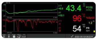
A parameter's  $\Delta x$ -value is displayed to the right of its online trend and corresponds to the difference between its current reading and its reading x minutes ago. x is called 'Delta-Time' and is adjustable between 1 and 120 minutes within a passwordprotected area of V-STATS<sup>TM</sup>. The default value for 'Delta-Time' is 10 minutes.
