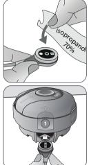
**1.** Verify that the sensor is clean before changing its membrane. If necessary, carefully wipe off any residue from the sensor's surface (including membrane, housing, groove and cable) with 70% isopropanol (for other approved cleaning agents refer to www.sentec.com/ifu).
