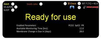
**Note:** Pressing the Enter Button (p. 55) while the 'Ready for use' screen displays activates a 'Quick Access Menu' with the possibility to activate additional calibrations (p. 27), to access the sub-menu 'Profiles', or to activate the V-Check<sup>M</sup> Mode (p. <u>46</u>).
