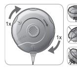
**b.** Turn the top portion one click clockwise to the next stop. Keep the Membrane Changer horizontal! Hold the changer's bottom half in place while turning the top half.
