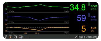
The RHP-reference value ('408' in this example) and the time that has elapsed since it has been determined/set ('00:16' in this example) are displayed underneath the RHP online trend. The dashed horizontal center-line in the RHP online trend corresponds to a RHP of 0 mW and reflects the RHP-reference value. RHP values below/above the center-line correspond to episodes during which the sensor required less/more power to maintain the sensor temperature than the AHP-reference value.
