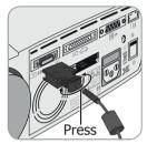
Connect the Digital Sensor Adapter Cable to the SDM. The connection is properly established when both clamps of the plug snap into place in the sensor connection port (15).
