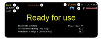
**Note:** Pressing the Enter Button (p. 44) while the 'Ready for use' screen displays activates a 'Quick Access Menu' with the possibility to activate additional calibrations (p. 16), to access the sub-menu 'Profiles', or to activate the V-Check<sup>TM</sup> Mode (p. 36).
