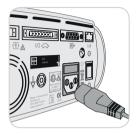
Plug the female connector of the power cord into the AC power connector on the rear of the monitor (23).
