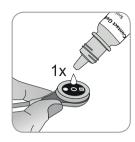
**8.** Apply **one small** drop of contact liquid to the center of the sensor surface. Ensure to keep the sensor horizontal (membrane pointing upwards) so that the contact liquid does not run off the membrane. Flip over the sensor just before inserting it into the ring.
