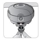
Press one last time or lift the sensor and remove it from the Membrane Changer. The  $\sqrt{\phantom{0}}$  symbol indicates that the membrane change is completed.
