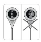
a) Change the sensor membrane if it is damaged or missing, has a loose fit, or if there is trapped air or dry electrolyte under the membrane.
