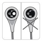
c) When operating with an OxiVenT<sup>™</sup> Sensor, **do not use** the sensor if the off-centered, white, round spot on the sensor surface is missing or is not illuminated in green-cyan color when the OxiVenT<sup>™</sup> Sensor is connected to the SDM with enabled PO<sub>3</sub> measurement function.
