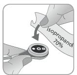
**3.** Clean the sensor with a swab wetted with 70% isopropanol to remove any contact liquid residues or dirt (for other approved cleaning agents refer to sentec.com/ifu).
