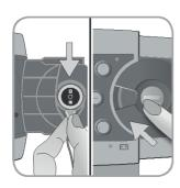
**5.** To calibrate the sensor, open the Docking Station Door and hang the sensor in the holder inside the Docking Station Door (the red light will appear). Close the Docking Station Door.
