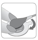
**2.** Place a finger on each side of the ring and rotate the sensor towards the index finger. The index finger will act as a wedge and will disengage the sensor from the ring.
