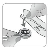
**1.** Verify that the sensor is clean before changing its membrane. If necessary, carefully wipe off any residue from the sensor's surface (including membrane, housing, groove and cable) with 70% isopropanol (for other approved cleaning agents refer to sentec.com/ifu).
