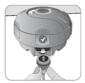
Press one last time or lift the sensor and remove it from the Membrane membrane that the change completed.
