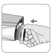
Insert the new gas bottle by turning it clockwise approx. 4.5 turns and thoroughly tighten it (without applying undue force).
