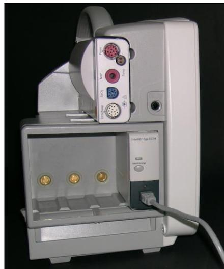
6. Connect the VueLink Adapter / EC5 ID Module to the SDM serial data port (use the screws to fix the Adapter / EC5 ID Module to the SDM). **Note:** Picture shows old type of VueLink Adaptor.
