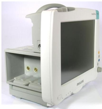
3. Insert the VueLink or IntelliBridge Interface Module in the module rack of the Philips Monitor
