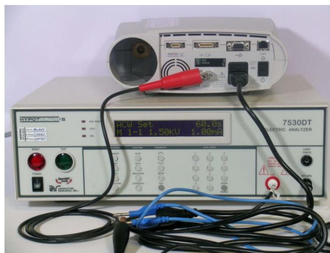
Figure 7 Connections for the High Potential Test, AP
