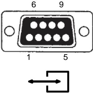
Figure 18 Serial Data Port (RS-232)
