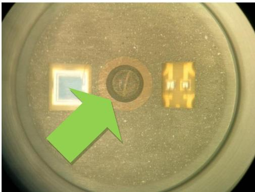
The sensor has an intact brown ring around the pH-glass.
