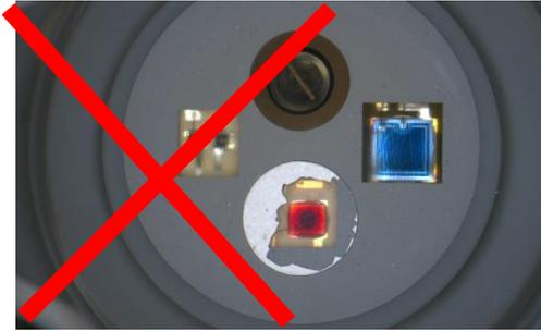
The white oxygen sensing spot is defect. This sensor needs to be replaced
