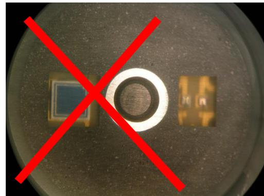
The ring around the pH-glass is intact but has a metallic luster, this sensor needs to be replaced
