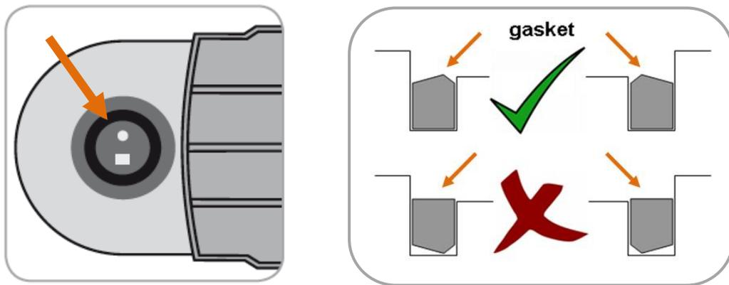
**Figure 9** Correct orientation of the Docking Station Gasket
