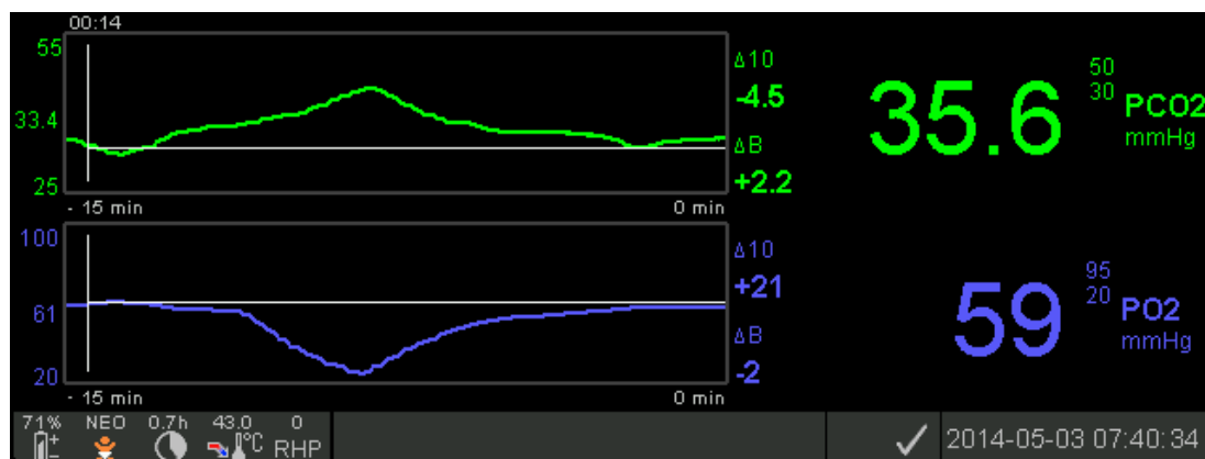
Figure 4 Example of a Measurement Screen with Δx-/baseline values
